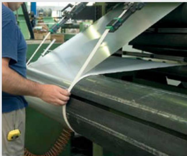
LV winding system
