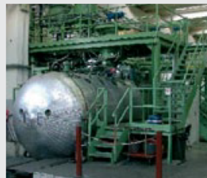
The pouring system under high vacuum.
